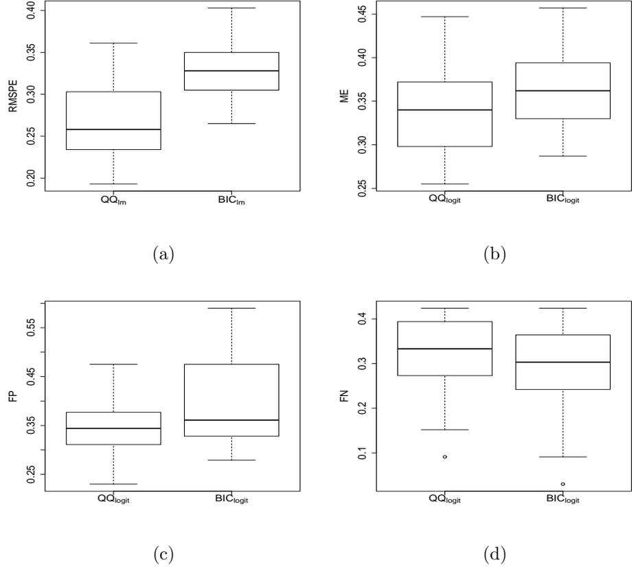
Figure 2: Comparison of Prediction Accuracy of the QQ Models and SMBIC for the Lapping Process: (a) Root mean squared errors (RMSPE); (b) misclassification error (ME); (c) false positive classification error (FP); (d) false negative classification errors (FN).
