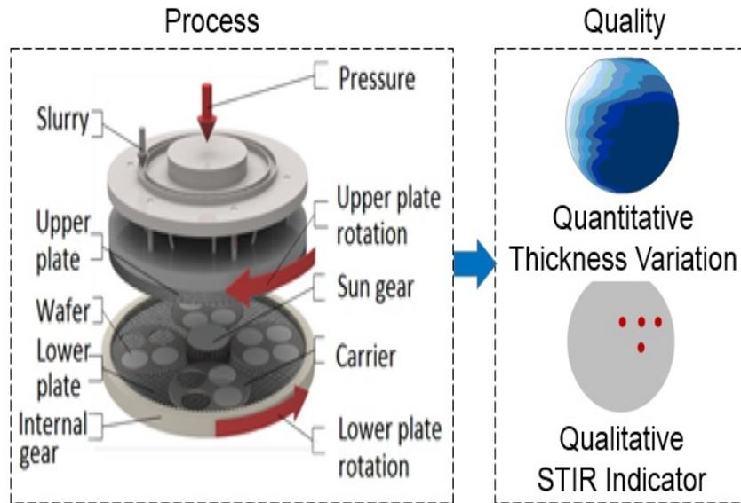
Figure 1: An Illustration of A Lapping Process with QQ Responses (Redrawn from Ning et al., 2012, and Zhao et al., 2011 with Authors' Permission).
